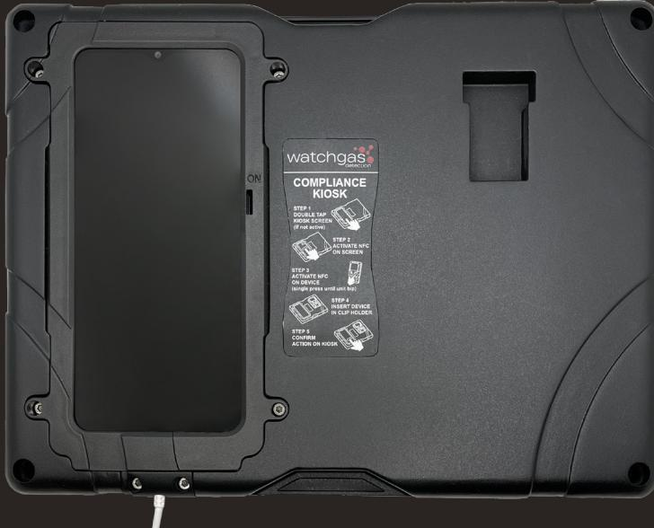
The WatchGas Compliance Kiosk works as a terminal to allow the user to check in the gas detector providing a full overview of the device status and any unforeseen events. The WatchGas compliance Kiosk automatically sends all data to a designated software site. This provides a cost effective overview of fleet health, predictive maintenance, events and alarms.
